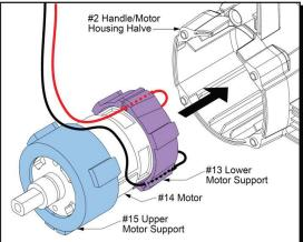
When reinstalling a new Motor Assembly, be sure that the red and black motor leads are fed through the large opening in the back of the Lower Motor Support before soldering wires to the On-Off Switch.
