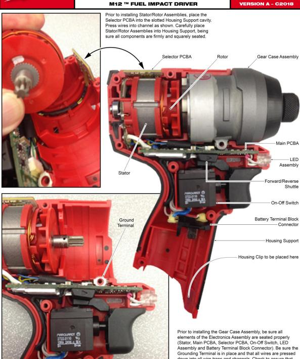
down into all wire traps and channels. Check to assure that wires will not interfere with moving parts.
