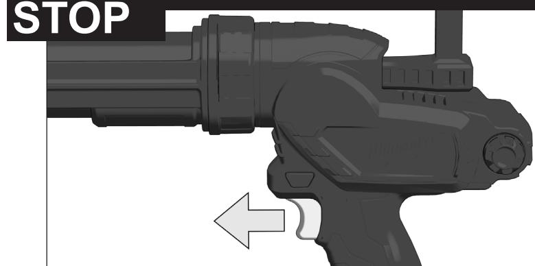
When the trigger is released, the motor will run for a short time to release the rod. This prevents a drip.
