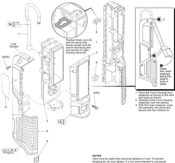
tools, hand tighten only. Torque screws #4 to 0.57-0.79Nm (6-8 kg/cm). Torque screws #10 to 0.34-0.45Nm (3.5-4.5 kg/cm).
