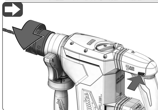
Operate the forward/reverse switch only until the product comes to a complete stop.
